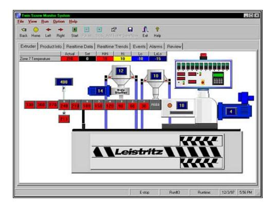
As you can see the data strip displays information from the Realtime Data page for the selected parameter. This allows you to see the alarm values along with the actual parameter value, and in the case of a temperature control zone, the temperature setpoint. Once the data strip is in view you can left click on any parameter and it will be displayed in the data strip.
