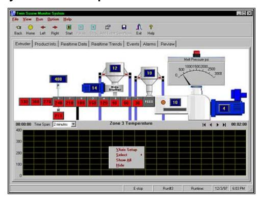
The Leistritz Twin Screw Monitor System (TSMS) is a powerful data acquisition software package designed to operate with the complete line of Leistritz Twin Screw extruders. The system monitors and archives all process parameters of your operation including:
