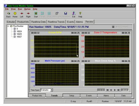
When you release the mouse button the graph window will re-scale based on the span of the dashed lines. This zoom feature differs from the zoom feature of the Extruder and RealTime Trends pages in that it re-scales both the x & y-axis.
