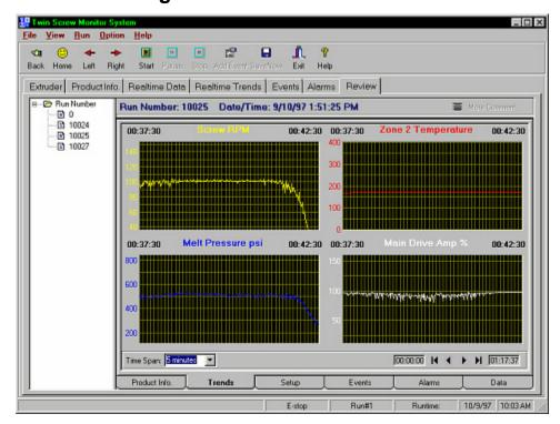
The Data Review Trends page allows you to view a graphic representation of your data. There are a number of tools available to assist you in customizing the graphic window for the best view of a selected parameter. To gain access to these tools place the mouse pointer in the plot area (black area) of the Trends window and click the right mouse button. The graph window popup menu will appear as shown below.
