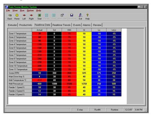
The Realtime Data page provides a digital snapshot of all process data, along with alarm limits for each parameter. Notice that the data displayed in the Actual column is color coded according to the current condition of the parameter (i.e. if a parameter enters a Hi condition it will appear with a yellow background in the actual column. If a parameter enters a Lo condition it will appear blue and so on).
