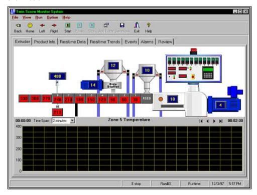
The graph view window contains tools for setting the time span of the graphic display and scroll buttons to allow you to pan through your test data. The figure below shows the location of these graphic tools.
