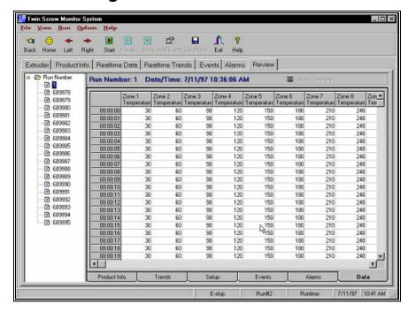
The Data Review Data page displays digital data from a run. The data on this page is displayed in a block of 300 data points. You can set the start time and the time increment for the data block by right clicking on the data table and selecting Data View Setup. The Data View Setup dialog will appear as shown below.
