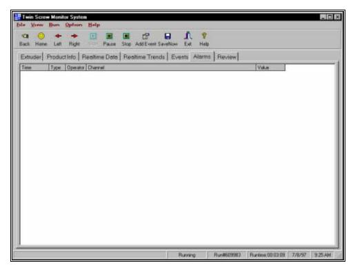
As we discussed earlier, you can set alarm values for each process parameter on the Realtime Data page. If a process parameter enters a Hi or Lo alarm state it will automatically be logged on the alarm page. Also, if a parameter progresses from Hi to HiHi or Lo to LoLo it will also be logged on the Alarm page. This information is also stored in your data file for future reference. The following information is logged on the Alarm page:
