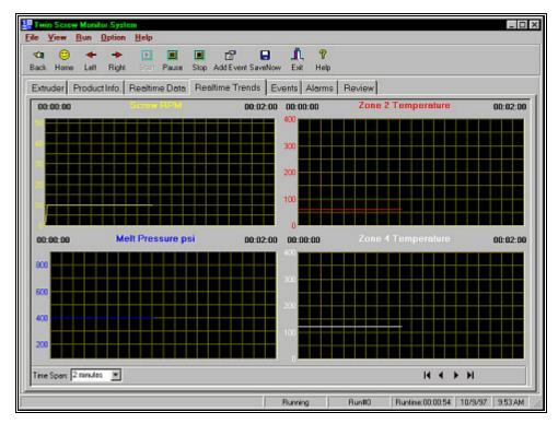
The Realtime Trends page provides a graphic display of 4 process parameters. These plots can be expanded to a full screen overlay view. The full screen (expanded) view can be used for easy comparison of real time trends.
