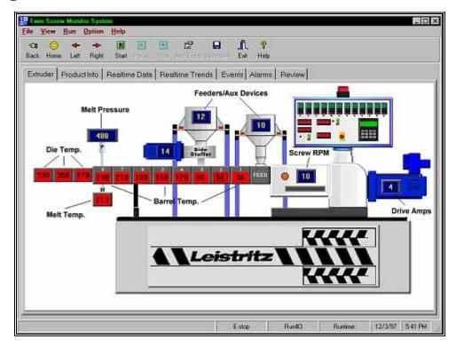
The Extruder page is the opening screen, which is presented when you first start the TSMS software. This page provides an overview of your complete process. The Extruder page provides you with information on:
